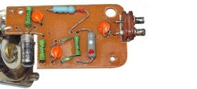
Bottom view of PCB with typical USSR manufactured components and brass tuning assembly.
